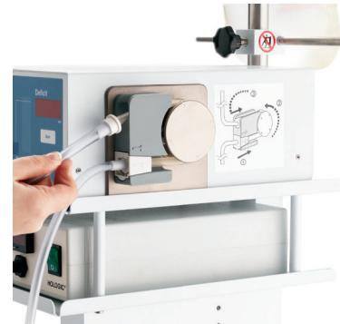
When prompted insert the inflow tubing around and past the roller wheel to secure into place.
