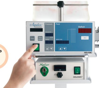
Turn on the Aquilex system before any tubing is connected to the roller wheel. The system will perform a self-diagnostic test.
