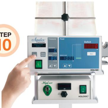
To prime the system check that the inflow stopcock is completely open and your fluid bag is unclamped.
